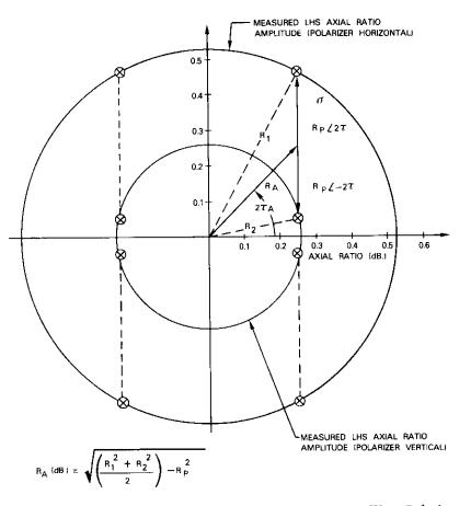
Figure 6. Polarization Diagram with Error Effects of Quarter-Wave Polarizer
