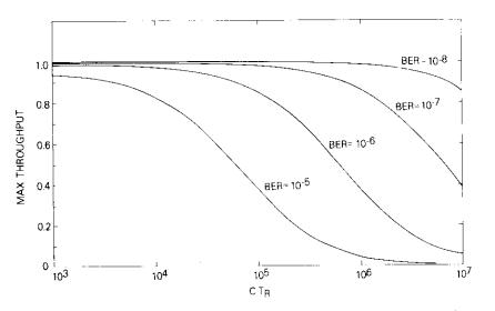
Figure 14. Maximum Achievable Throughput for HDLC FDX-NRM
