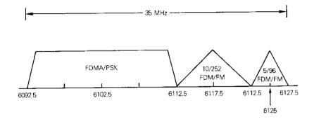
Figure 13. Frequency Plan for Example 4
