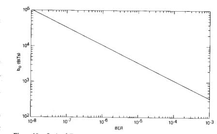
Figure 10. Optimal Frame Length  $(b_0)$  vs Bit Error Rate (BER) for HDLC HDX Mode (frame overhead, A = 56 bits)
