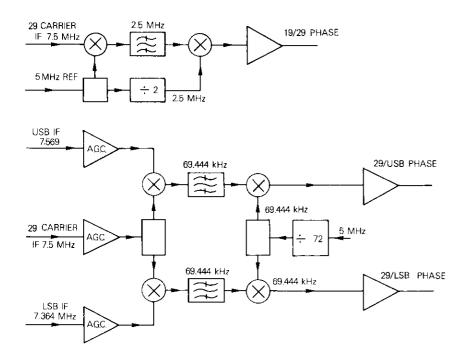
Figure 8. 19- and 29-GHz Phase Detectors
