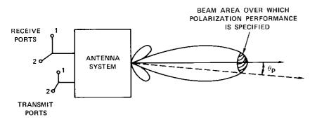
Figure 2. Basic Port Configuration of Dual-Polarized Earth Station Antenna
