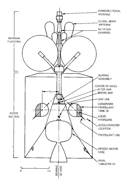
Figure 3. INTELSAT IV Spacecraft with Cutaway View of Rotor Section
