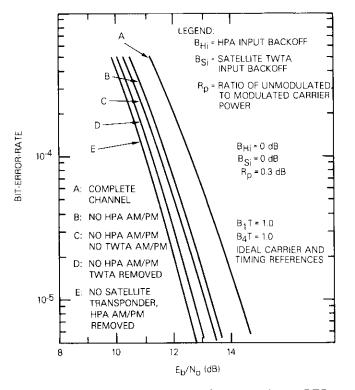
Figure 7. Effect of Component Characteristics on BER
