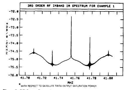
Figure 8. RF Power Spectral Density of the Intermodulation Noise at the Input of the Receiver of the SCPC Carrier at XX41.755 MHz
