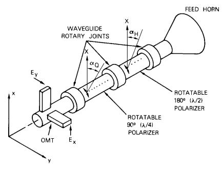
Figure 11. Circuit for Measuring Polarization State
