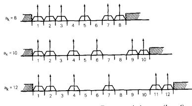
Figure 4. Examples of Optimum Frequency Assignment (k = 6)
