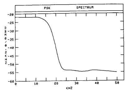
Figure 7. Measured SCPC/PSK Power Spectral Density
