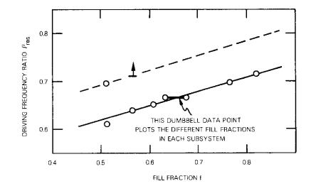
Figure 9. Driving Frequency Ratio at an Anomalous Resonance vs Fill Fraction for the Conispheric Tanks
