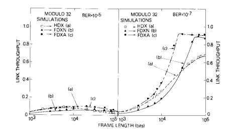
Figure 9. Model and Simulation Comparisons for a 1.544-Mbit/s Satellite Data Link
