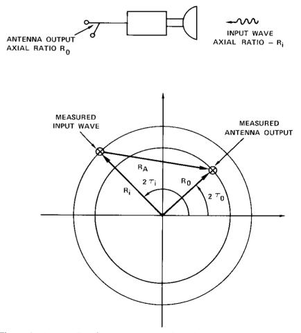
Figure 4. Antenna Depolarization Expressed as the Vector Difference of Input and Output Polarization States
