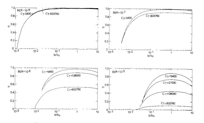
Figure 22. Frame Length vs Maximum Throughput Tradeoff for FDX-ARM
