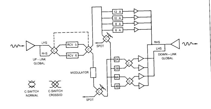
Figure 7. Simplified Block Diagram of INTELSAT IV-A F2 and F3 Dual Polarization Transponder
