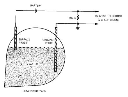
Figure 10. Liquid Height Gauge Circuit for Liquid-Slosh Quantitative Measurements
