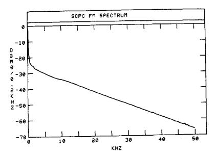
Figure 6. Power Spectral Density of SCPC/FM Carriers
