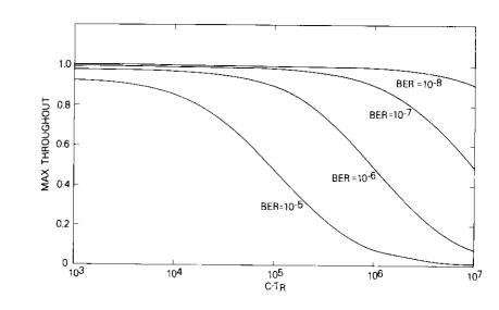
Figure 16. Maximum Achievable Throughput for FDX-ARM
