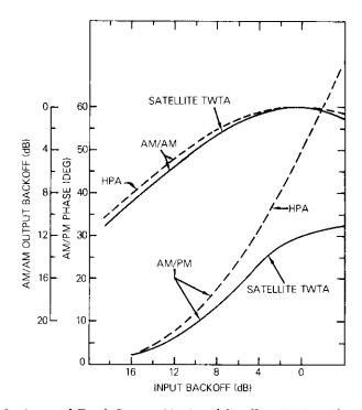
Figure 3. Assumed Earth Station HPA and Satellite TWTA Characteristics
