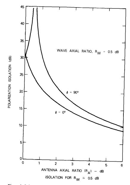
Figure 3. Polarization Isolation vs Antenna Axial Ratio for a Wave with 0.5-dB Axial Ratio
