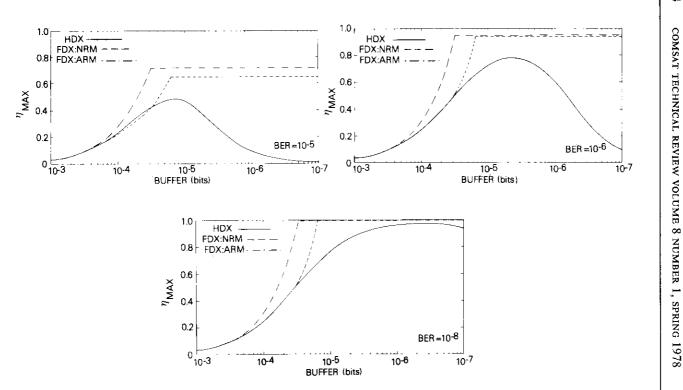
Figure 25. Maximum Throughput vs Buffer Size for a 56-kbit/s Satellite Channel
