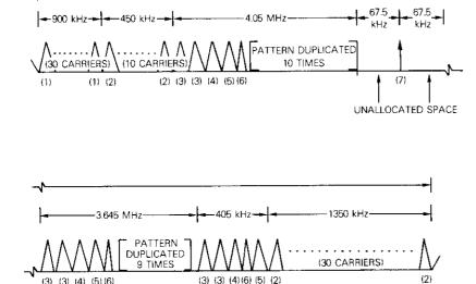
\* NOTE THAT THE FREQUENCY PLAN SHOWS THE AVAILABLE CHANNEL BANDWIDTH SLOTS. NOT ALL OF THE SLOTS ARE OCCUPIED SIMULTANEOUSLY. AN ACTIVITY FACTOR OF 40% FOR 160 CHANNELS WAS ASSUMED.
