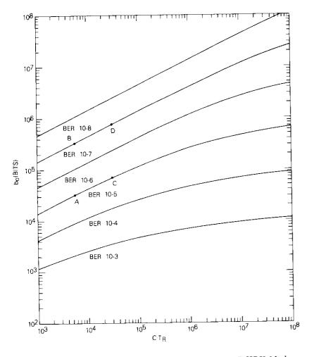
Figure 11. Optimal Buffer Size  $(B_0)$  vs  $C_T$  for HDLC HDX Mode (A = 56 bits)
