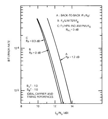
Figure 8. BER Performance with Modem Filters Only, with a Hard Limiter, or with an HPA without AM/PM
