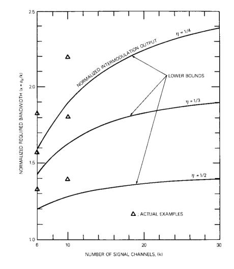
Figure 3. Required Frequency Bandwidth vs Number of Signal Channels
