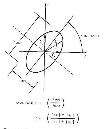
Figure 1. Definitions for Elliptically Polarized Wave
