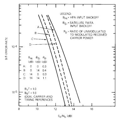
Figure 6. BER Performance for the Complete Transmission Link (all components included;  $B_1T = 1.0$ ,  $B_4T = 1.0$ )
