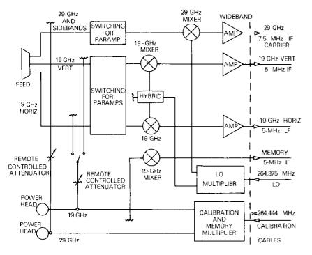
Figure 1. RF Head Block Diagram
