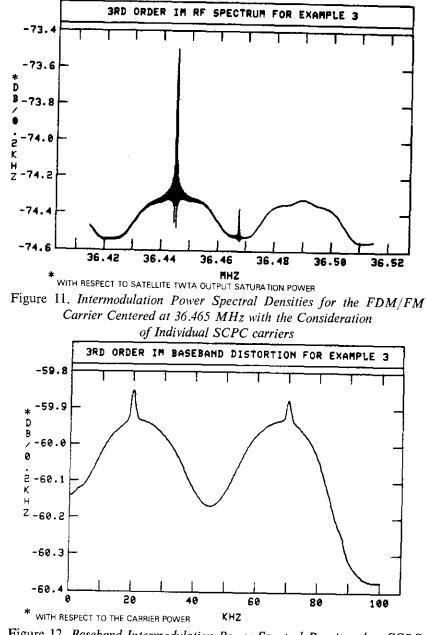
Figure 12. Baseband Intermodulation Power Spectral Density when SCPC Carriers are Individually Considered
