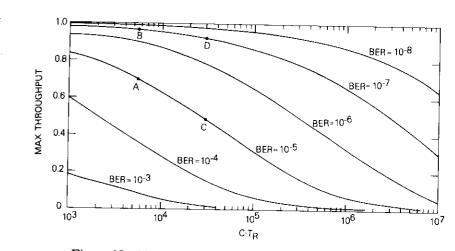
Figure 12. Maximum Achievable Throughput vs C  $T_R$  for HDLC HDX Mode (A = 56 bits)
