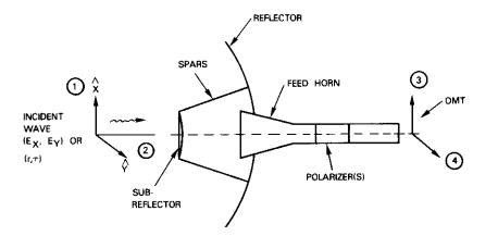
Figure A-1. Antenna Geometry and Depolarizing Mechanisms
