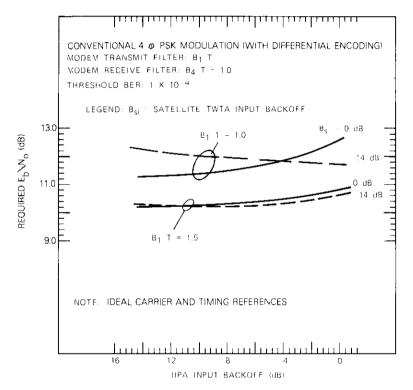
Figure 5. Effect of HPA and TWTA Backoff (modem transmit filter  $B_1T$ product,  $B_4T = 1.0$ )
